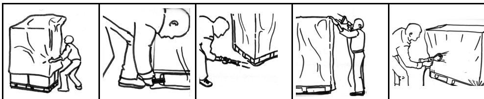
The four corners of the pallet to be shrink-wrapped must be free, and therefore pallets must be raised using another pallet, or better still, a robust support.
